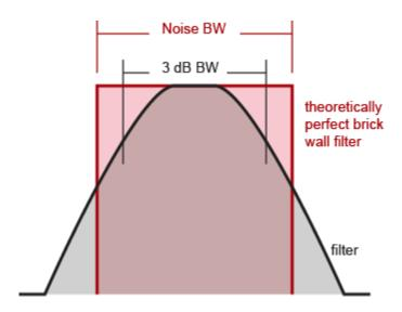
Noise bandwidth is ALWAYS wider than 3 dB bandwidth, because there's still filter left beyond the 3 dB points. The more poles the filter has, the steeper the sides, and the closer the noise bandwidth is to the 3 dB bandwidth. Since a perfectly rectangular filter is not possible, the noise bandwidth is always wider than the 3 dB bandwidth.
